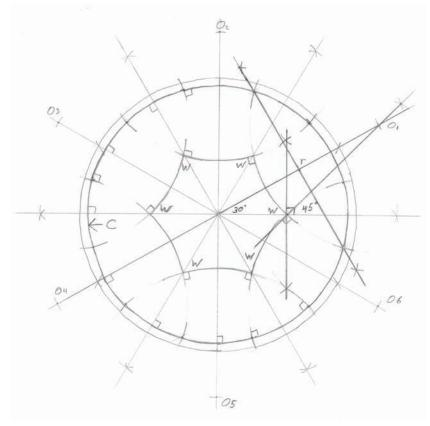
This is the first step, so to speak, in the construction of Escher's "Angels and Devils." Eight wing tips meet at each point marked with a "W," and these points along with the center and the circumference "C" of the circle are in correct proportion to each other. The key in dividing the various segments is in the use of orthogonal arcs.
